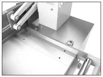
Figure 15. Fence mounted to table.
